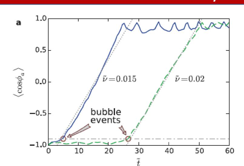
Bubbles appear via quantum tunnelling (t = 5, v = 0.015 and t = 26 v = 0.02) and grow with the speed of sound.
