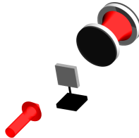
Figure 1: Coupling light interacting with a cantilever to a cavity enhances the optomechanical friction force by several orders of magnitude.
