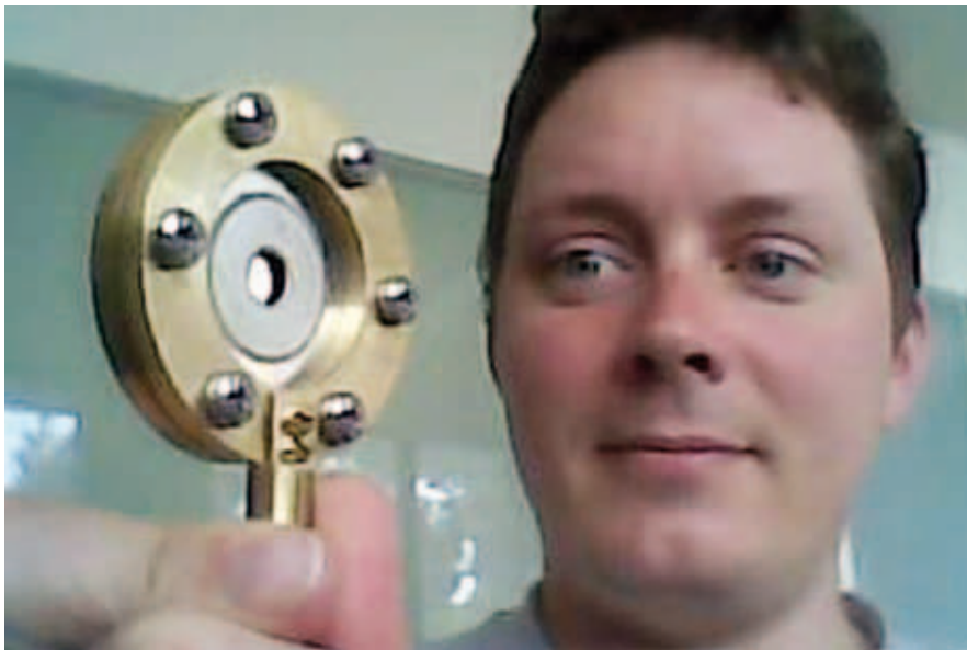
Wilfred holding an ultrasonically driven miniature bubble chamber being prototyped for use with ultrashort pulsed X-ray sources.
