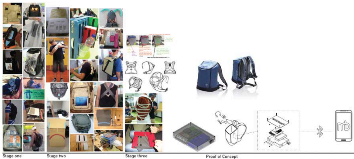
A timeline of the three stages in physical prototyping running from the start of the process to the proof-of-concept
