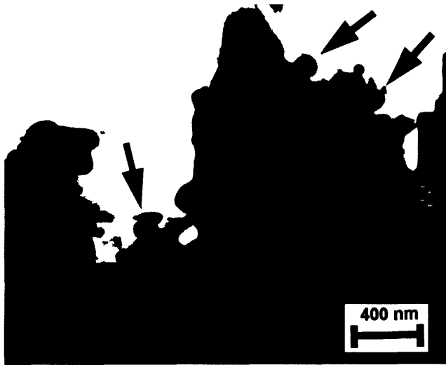
Fig. 9. TEM image of a zirconia specimen heat-treated at 1273 K for 1.0 h.
