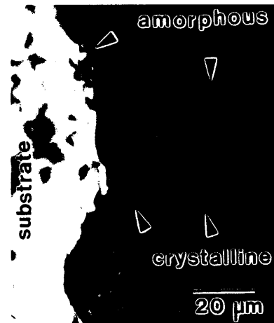
Figure 7. A polished cross section of a hydroxyapatite coating exhibiting the amorphous phase (dark gray) and crystalline phases (light gray). The white area to the far left represents the substrate. The magnification bar is 50 \mu\text{m} wide.
