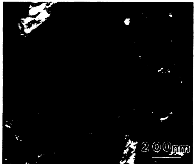
Fig. 31 Dark-field image of methanol-milled Ni cross-sectional (10 h) coating
