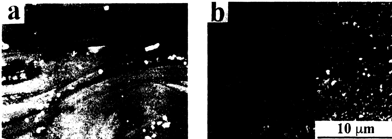
Fig. 9 Scanning electron micrographs of sprayed deposits containing 2.0 wt% B. (a) As-sprayed deposit. (b) Deposit heat treated at 1173 K for 2 h
