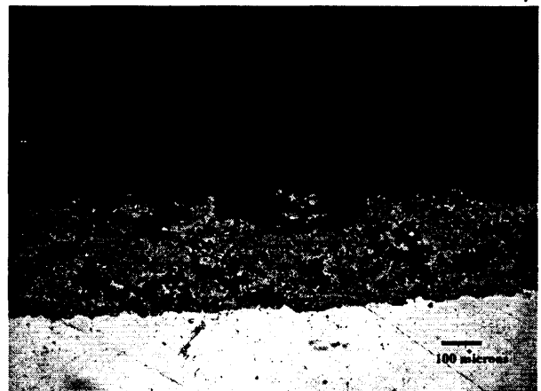
Figure 12. Cross sections of plasma sprayed X-form 205 on tube ends at 25X and 50X magnification.
