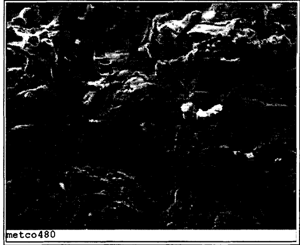
Figure 8. SEM micrographs of Metco 480 surface at 100X and 500X magnification.
