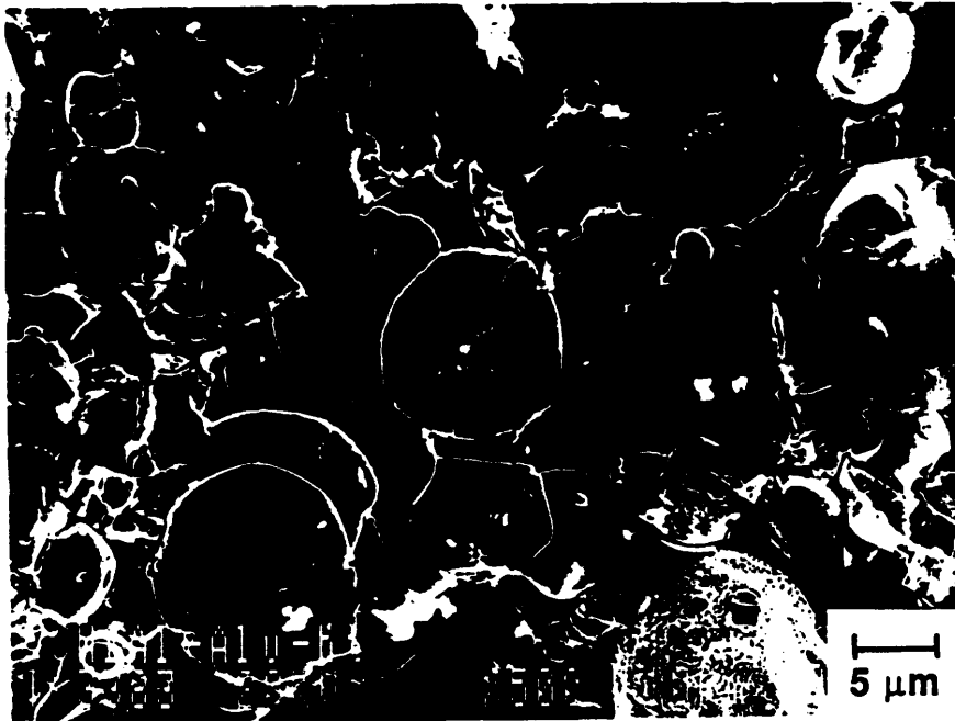
Figure 2. Surface features of a well-melted ceramic coating.
