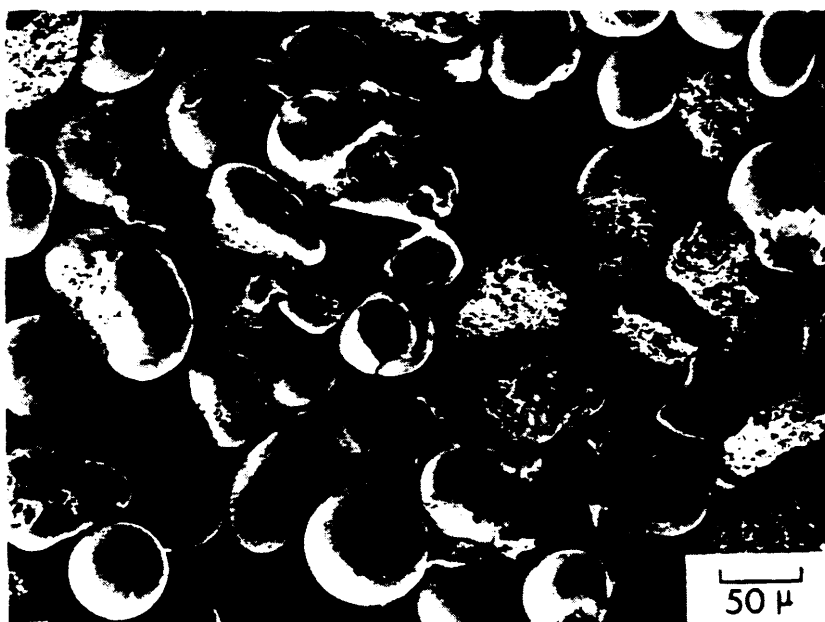
Figure 40.6 Plasma-spray quenched 8 wt. % Y 2 O 3 -ZrO 2 powder. Note the intricate topology and partial melting of some particles.
