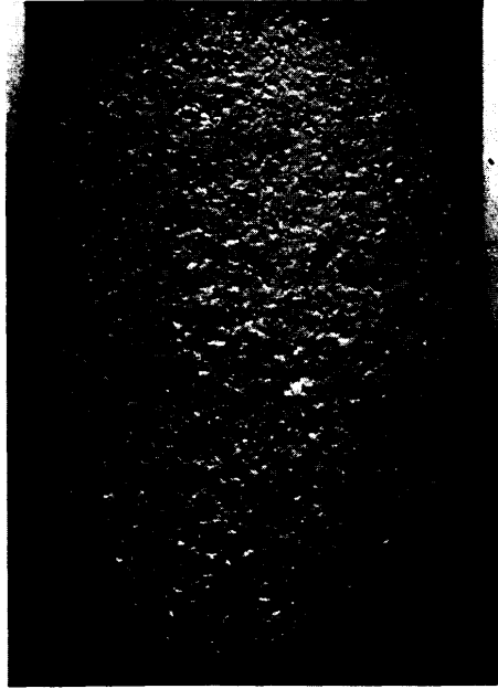
Fig. 5. As-sprayed \text{ZrO}_2\text{-8wt.\%Y}_2\text{O}_3 specimen after 15 cycles of 2.5 s (case B) in a 30 kW plasma flame.
