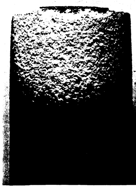
Fig. 7. Laser-glazed \text{ZrO}_2\text{-8wt.\%Y}_2\text{O}_3 specimen after the first 25 of a total of 1000 cycles of 0.5 s (case E) in a 30 kW plasma flame. The hot zone is near the bottom. Edge effect cracking of the coating occurs on the hollow specimen in the unglazed region near the top.
