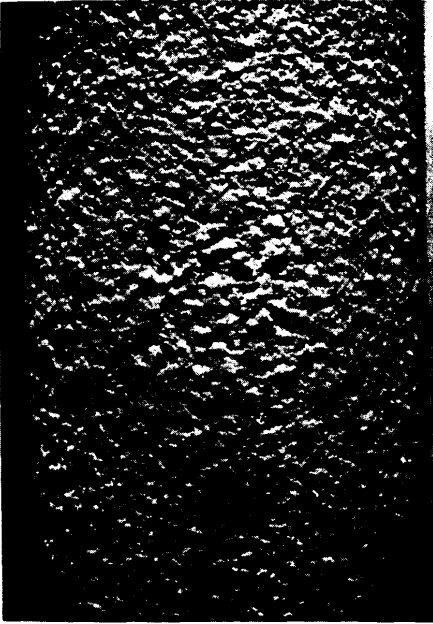
Fig. 5. As-sprayed \text{ZrO}_2\text{-8wt.\%Y}_2\text{O}_3 specimen after 15 cycles of 2.5 s (case B) in a 30 kW plasma flame.
