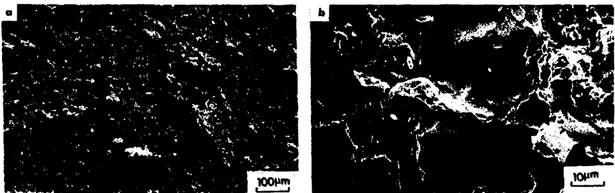
Fig. 4. Cohesive fracture of as-sprayed stainless steel coating: (a) Area revealing interlamellar tearing; (b) magnified image indicating ductile fracture.
