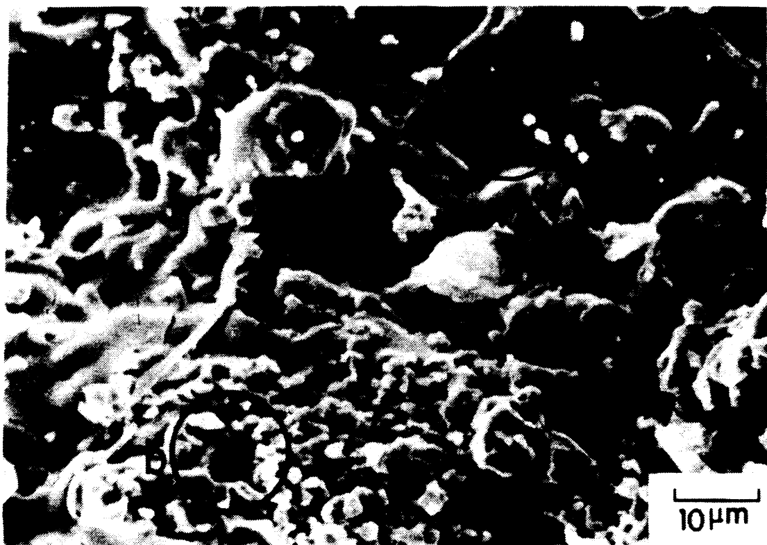
Fig. 4. Surface of plasma-sprayed YSZ coating showing regions of fine cracks (region "a") and unmelted particles (region "b").
