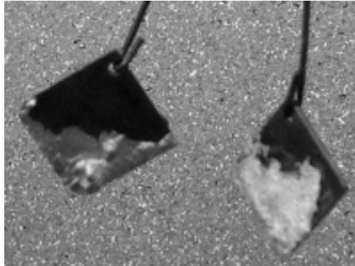
Figure 2 - Example of samples after removed from the AZ91D Melt
