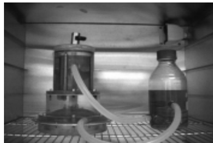
Figure 1 - Set-up of bioreactor (left) in a standard humidified incubator at 37°C and 5% CO 2 , connected to a reservoir (right) for CO 2 -exchange.
