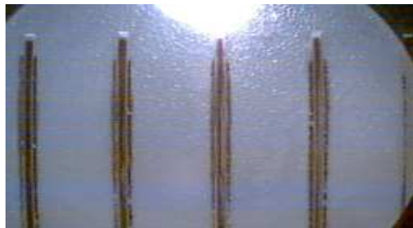
Figure 3.1 - Laser-ablated microchannels in polycarbonate. Channels are 400 \mu\text{m} wide, 17mm long and vary between 38 and 200 \mu\text{m} deep. The channels are separated by 5mm.
