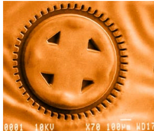
Microgear mould laser ablated into 60 micron thick SU-8. Aspect ratio 4.5
