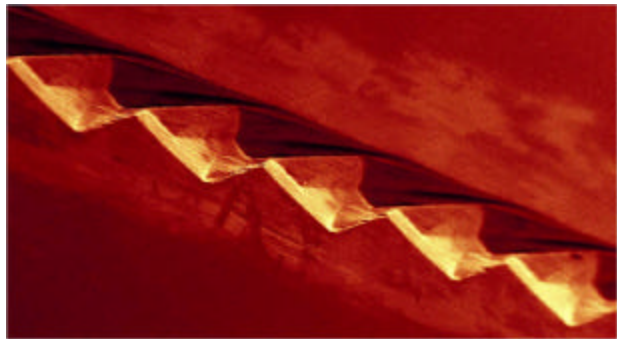
A structured fluidic channel 70 micrometers wide used to create turbulent flow.
